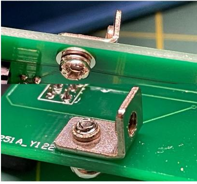
Your expansion bus circuit board is complete and may be plugged into the main unit. Be sure to have the brackets sit behind the clear acrylic back. Wiggle the expansion board back and forth to get it to sit firmly in the shrouded male header. Secure it in place with two 6mm M3 bolts
