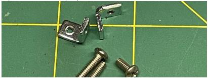
The two side of the L-bracket are slightly different. Attach the longer side to the bus circuit board with an M3 bolt, trying to make it as square as you can.
