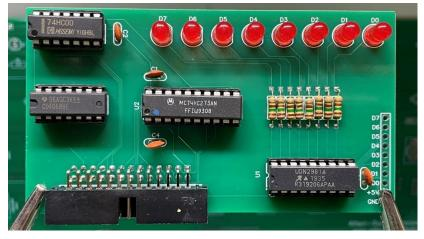
Your LED Output Register expansion card is complete and may be inserted into any slot on the expansion bus.
