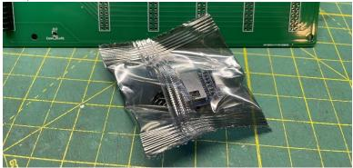
You will need to solder the male header to the SD card module. It is very important you install the header as pictured, and solder it to the circuit board as pictured:
