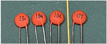
The 104 capacitors go in locations C1, C2, and C3. The 471 capacitor goes in location C4.
