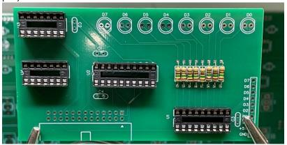
Add the eight LEDs next, with the long lead in the left hole and the flat part of the LED to the right.
