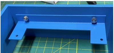
Turn the assembly over and it should look exactly like this. Note the placement of the mounting holes.
