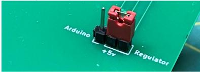
In general, you should select "Regulator" which provides power from the L7805CV regulator, but this will only provide power when the kit is powered from a plug-in 9-12v power adapter (included.) Selecting "Arduino" will power the cards from the Arduino's internal regulator. That means power will be available when the kit is powered from a USB connection, but this power supply is limited and may not be sufficient for multiple expansion cards.
