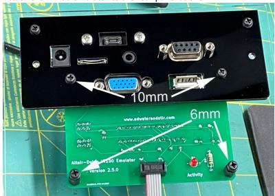
Secure it with two 6mm nylon bolts on the bottom and two 10mm nylon bolts at the top.
