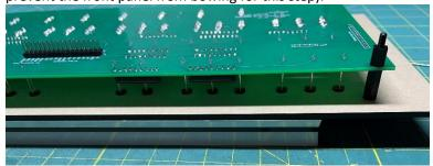
After you have soldered all LEDs, you can remove the front panel.
