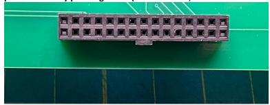
Add the 14-pin female header to the "Standard Exp Conn" (J1) area on the right side of the circuit board. This is installed on the **back** of the circuit board.
