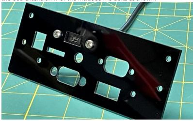
Take the clear acrylic pane and peel the protective plastic from both sides. Attach the rear ports panel with two 10mm M3 bolts and two nuts as shown in the photo.
