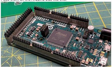
Insert the Arduino into the **back** of the main circuit board and solder all header pins in place (note: this is where most errors happen – it's easy to miss one or two header connections.)
