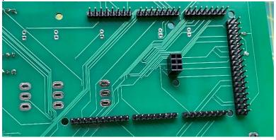
Add a 2x3 (six pin) male header to the rear side of the circuit board for the VT100 emulator connector.
