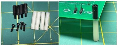
We're going to temporarily add the standoffs to the main circuit board with the 15mm on top and 20mm on the bottom (temporarily).
