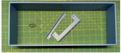
Place the aluminum frame with the holes closest to the top, and mount the smaller side bracket **exactly as shown**:
