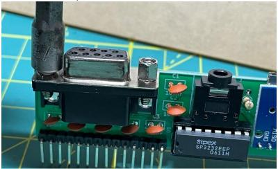
Attach the daughter board assembly to the rear port panel and secure with the jack nuts.
