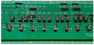
Be careful that you don't over-heat the toggle switches while soldering. This can damage the switch mechanism. Instead of soldering all three lugs on the toggle one after the other, I solder the top lugs on all switches, then the center lugs, then the bottom lugs like this:
