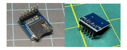
Solder the audio jack and SD module to the circuit board.
