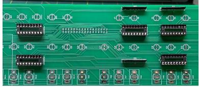
Add the 26-pin female header to the "Experimenter IO Bus Connector" (J6) area in the middle of the bottom of the circuit board. Be sure to install the header on the **back** with the
