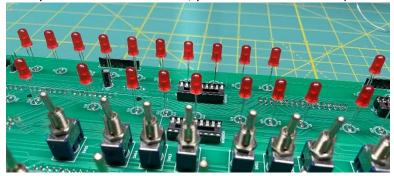
When you are done adding the LEDs, you can remove the 20mm standoffs and replace them with 8mm standoffs.
