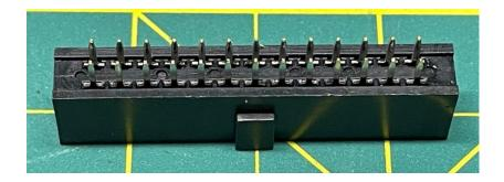
Solder all five 26-pin female headers and a three pin male header to the circuit board. **The orientation of the polarizing key on the female headers is critical**, make sure they face right as shown.
