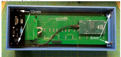
Apply the Altair 8800 sticker to the front panel. The adhesive is forgiving, so if you place it wrong, you can pull it up and put it in place again. Use a small Phillips screwdriver or awl to poke holes where the bolts will go.
