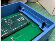
Plug the USB extension cable into the Programming Port on the Arduino Due (the port closest to the power jack.)
