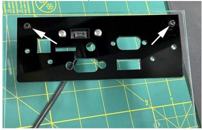
Remove the jack nuts from the DE9 connector. You can do this with a 3/16" driver or a pliers.
