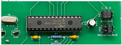
Baud rate jumpers are placed vertically over C and B (for 9600 baud) leaving A unjumpered. Place a monitor color jumper vertically, I prefer green.
