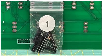
Add the five resistor arrays in RN1-RN5, making sure the dot indicator faces to the left side (where the square is on the circuit board) as pictured.
