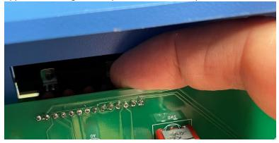
Secure the rear panel in place with two 10mm nylon bolts and two 6mm nylon bolts.
