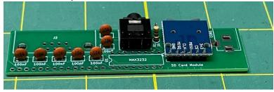
Add the DE9 connector, the power jack, and the DIP socket.
