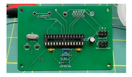
Turn the board over and mount the following components on the front:
