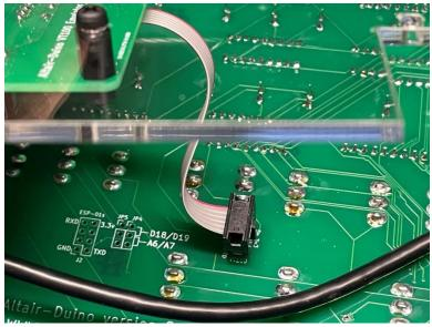
The next part can be somewhat tricky. You need to insert the 14-pin male header from the expansion circuit board into the 14-pin female header on the main circuit board.
