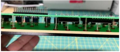
Then support the front panel while you solder the LEDs in place (to prevent the front panel from bowing for this step).
