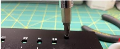
Flip the entire assembly over and allow the LEDs to fall into place in the front panel.
