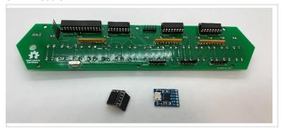
The DS3231 module simply mounts on the five-pin male header in the center, and the USB to UART module is soldered to the
