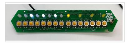
Remove the nut holding the power switch in place (if you used it) and place the acrylic cut spacer over the circuit board.
