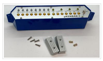
The pieces are held in place by 14mm flat head bolts and brass knurled nuts.
