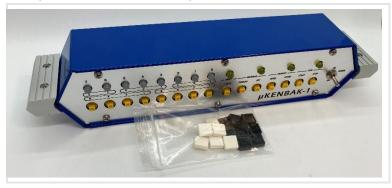
The button caps will fit in any orientation, but I have found that it's best to have the buttons mounted as pictured. It makes it easier to pry the buttons off (from the top and bottom) if necessary.
