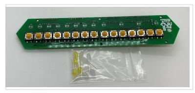
The orientation if the LEDs is crucial. Make sure the long lead of the LED is toward the right of the PC board and the flat side of the LED is toward the left (as indicated on the screen print.)
