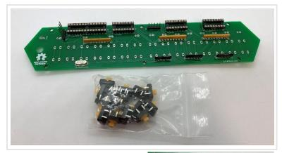
These will be placed on the front side of the circuit board (with the Adwater & Stir logo.) It is important that they are installed flat and aligned, so they will later align correctly with the front panel.
