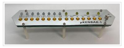
There are six M3 washers included with the kit. You may want to use these to increase the spacing between the circuit board and the front panel. I find they work well. If you use these washers, you will also want to use the lock washer for
